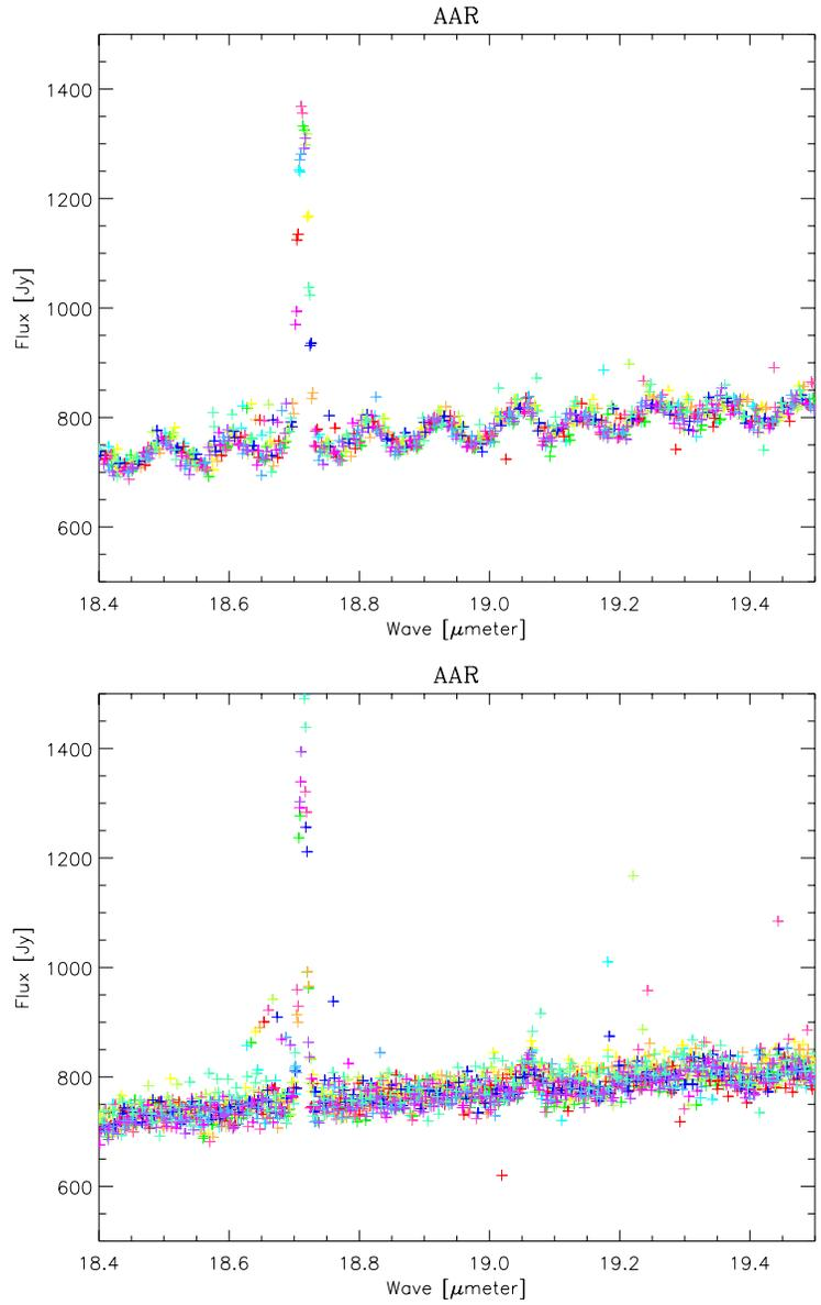
Figure 2: These figures show the utility of FRINGES. The top figure is the OLP10.1 AAR for a spectral fragment in AOTBAND 3C. The SIII forbidden line is quite evident. What is not so clear is the HI 8-7 line at 19.06  $\mu\text{m}$ . This line is clearly seen in the high resolution and defringed product.
